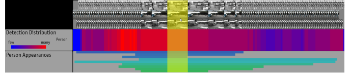
Figure 8. Bottom panel visualizations. The top element serves as a frame preview. In the center, a heat-map depicts where in the timeline many entities of the selected class (here “Person”) were detected. At the bottom, lines indicate, for each detection in the current frame, when it first appeared in the scene and when it disappeared again.
