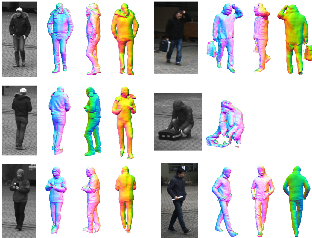
Figure 7. 3D models of different persons reconstructed from single images using PiFuHD. The reconstruction time was approximately 10 seconds per person. The size of the image patches varied between 260 \times 330 and 440 \times 960 pixels. Most models were successfully reconstructed from all sides. Only the kneeling man opening a suitcase (lowest resolution) could not be reconstructed from the back.
