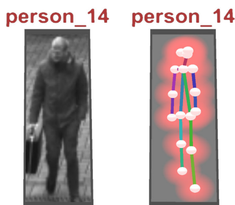
Figure 9. For each person recognized in a video frame ( Left ), OpenPose is applied for skeleton extraction. The extracted skeletons can later be displayed in the scene as connected points ( right ).
